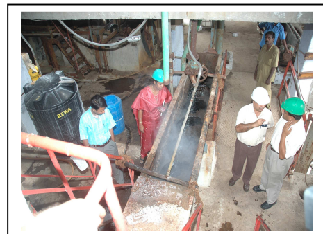
5. MC Pump & Standpipe installed at SPB to enhance enzyme mixing
