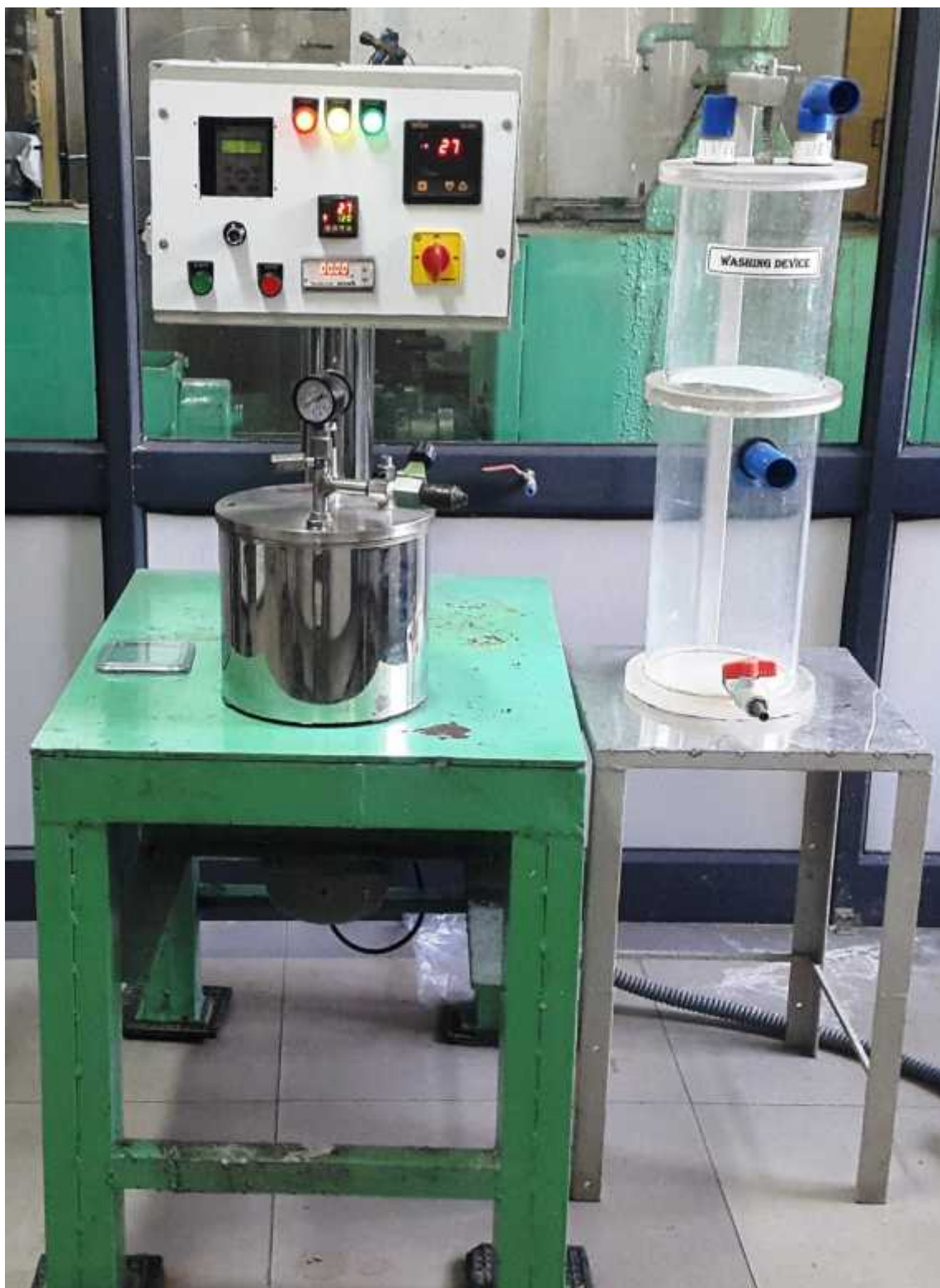
Figure 6.1.1: Oxygen bleaching reactor fabricated at ACIRD
